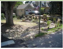
garden idea could be a good possible solution to this existing drainage problem. The soils in my rear yard are very good in terms of percolation. A percolation test in the existing soils revealed a 20 minute drain time of an 8" diameter hole! The problem was trying to collect the water from the parking lot/Town street area to this new rain garden area.
